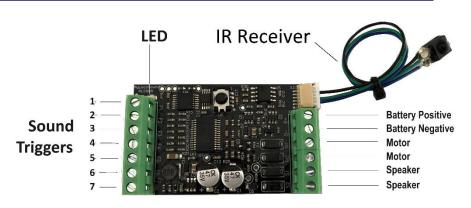
controller has the appropriate outputs available. The trigger terminals are labelled F1 to F7 and are referred to by these labels in these instructions e.g. "Triggering F1" means to close a contact between the F1 terminal and the Battery negative terminal.
