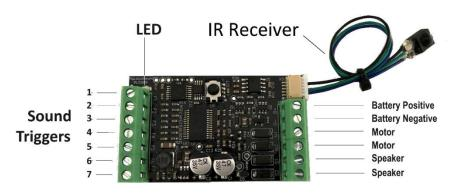
connections on the left trigger the various sounds where the locomotive controller has the appropriate outputs available. The trigger terminals are labelled F1 to F7 and are referred to by these labels in these instructions. For example, "Triggering F1" means to close a contact between the F1 terminal and the Battery negative terminal.
