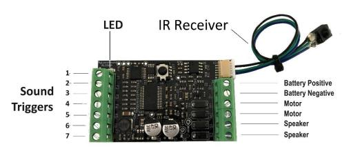
sounds where the locomotive controller has the appropriate outputs available. The trigger terminals are labelled F1 to F7 and are referred to by these labels in these instructions. For example, "Triggering F1" means to close a contact between the F1 terminal and the Battery negative terminal.
