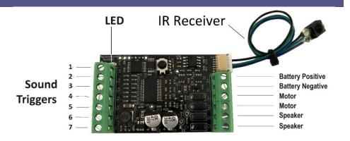
connections on the left trigger the various sounds where the locomotive controller has the appropriate outputs available. The trigger terminals are labelled F1 to F7 and are referred to by these labels in these instructions. For example, "Triggering F1" means to close a contact between the F1 terminal and the Battery negative terminal.
