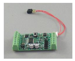
However, if the soundcard in the locomotive is completely enclosed then it will be necessary to use a tiny receiver on a small flying lead and to mount that receiver on the exterior of the loco motive in a position where it is hard to see, such as under the footplate.
