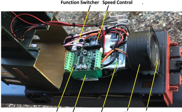
Soundcard Battery Pack Receiver Baffle Box Speaker
