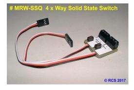
Each pair of function switches has a button on top which switches between momentary and latching operation. In momentary operation the switch is on for as long as you press the button on the transmitter and goes off as soon as you release a button. In latching operation, the switch goes on when you press and release the transmitter button and then stays on until you press and release the button again.
