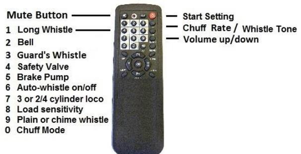
Adjustments to the sounds can then be made without taking the loco apart to access the soundcard.
