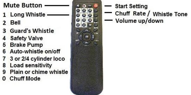
Note that the buttons on the MyLocoSound remote control auto-repeat if held down. If you want a single event to occur, like turning on the safety valve, then press the safety valve and release it immediately. If you want to make a large change in volume or tone then you can hold the button down to avoid the need to press the button repeatedly.
