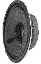
The lowest cost option is to fit a speaker from your local consumer electronics store. Typically these come in 27mm or 57mm diameters. Use the largest which you can fit in your loco.
