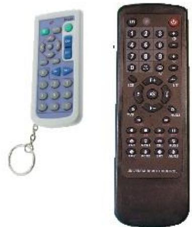
The remote control communicates with the soundcard via two infra-red receivers. One is located on the soundcard and the other is on a flying lead which allows it to be fixed to any external surface of the loco. Adjustments to the sounds can then be made without taking the loco apart to access the soundcard.
