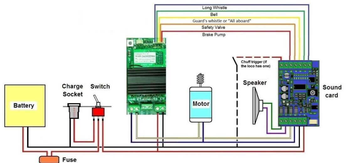
A chuff switch can be set up on the tender or van wheels. The soundcard automatic modes can be used to make a whistle sound on departure and at timed intervals. Other sounds can also occur automatically using the modes provided. A rechargeable PP3 battery should sustain continuous running with an automatic whistle for about two hours.
