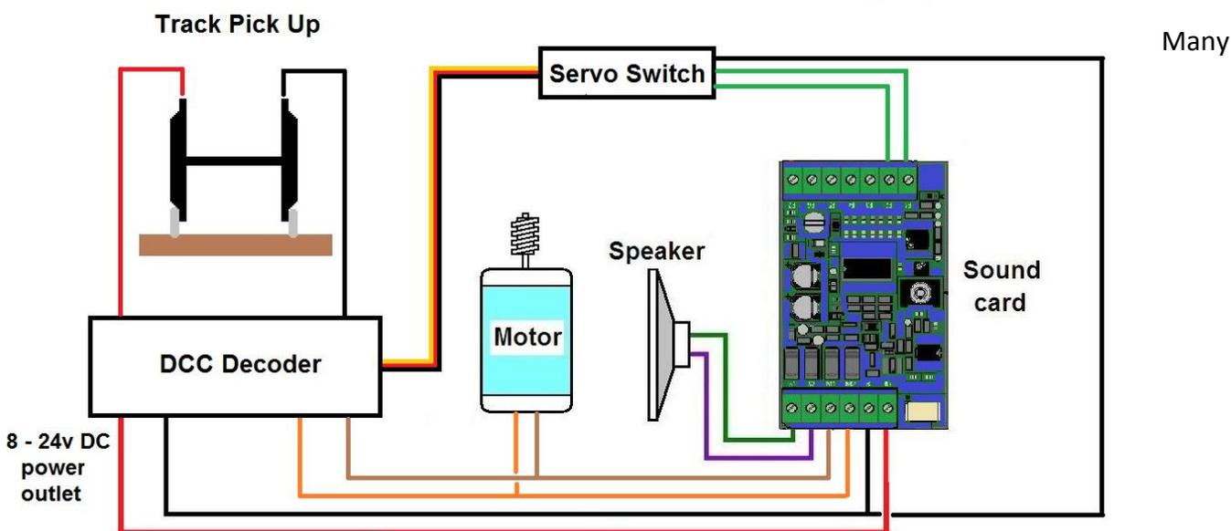
decoders also have function outputs which can be used to trigger sounds. However, this is technically difficult and you should only attempt it if you are very familiar with your decoder and the setting of CVs.
